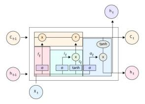
Fig. 1. LSTM model structure
